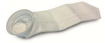
The no-bypass welded seams eliminate the possibility of fluid bypass through needle holes. We provide a variety of glazed and singed finishes to inhibit fiber migration. FSI also offers polyester inserted felts. These inserted felts include a reinforcing scrim needled inside the felt material, to provide added strength and durability, when a restrainer basket is not being used.
