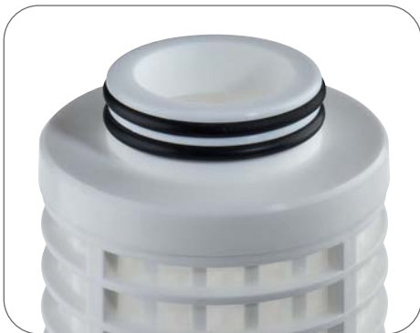
BX - Quick-fit configuration with 45 mm double o-ring end-cap.
