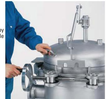
6. Close the V-clamp by rotation of the spindle
