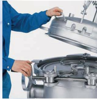
3. Open the cover aided by spring assisted mechanism
